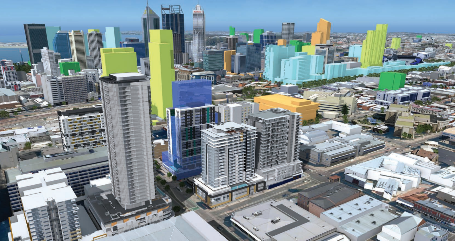
Example of the 3D City Model with DA model submissions in the foreground.
